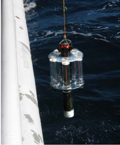
Neutrally Buoyant Sediment Trap being lowered into water from RV Kilo Moana off Hawaii. (Photo by Ken Buesseler, Woods Hole Oceanographic Institution)
