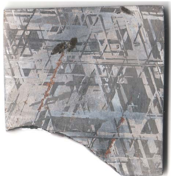
This slice of the Gibeon IVA iron meteorite, 4.6-centimeters wide, displays a Widmanstätten pattern. (Photo by Jeff Gillis-Davis, University of Hawaii)
