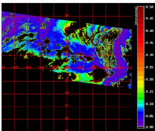
Figure 1. Aerosol optical depth (870 nm) calculated from a SeaWiFS image using the SeaDas software.
