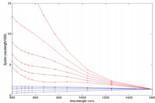
Figure 4. Aerosol single scattered radiance (at 135 degrees scattering angle) normalized by the aerosol single scatter radiance at 1600 nm.
