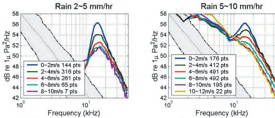
**Figure 3.** The average sound spectra for rainfall rates of 2-5 (left) and 5-10 (right) mm/h are decomposed into various wind speeds. **Gray area**, wind-only spectra; **dashed-dotted** (left), **dotted** (center), and **dashed** (right) black lines, average spectra for wind speeds at 2-4, 4-6, and 6-8 m/s, respectively; **numbers in box**, number of data points in each category (Ma and Nystuen, 2005b). Increasing wind speed causes decreasing sound levels in a predictable way.
