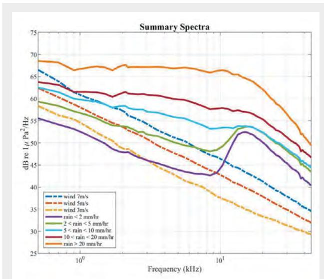
**Figure 2.** The spectra of ambient sound during times of only rain or only wind. The data were collected from 14 open ocean locations over 90 months (Ma and Nystuen, 2005a), © American Meteorological Society, used with permission.
