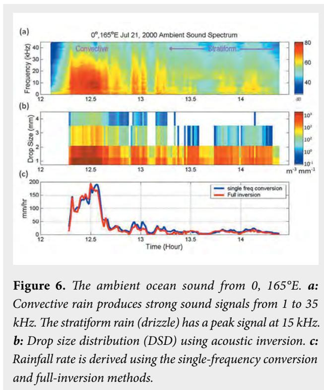
**Figure 6.** The ambient ocean sound from 0, 165°E. **a:** Convective rain produces strong sound signals from 1 to 35 kHz. The stratiform rain (drizzle) has a peak signal at 15 kHz. **b:** Drop size distribution (DSD) using acoustic inversion. **c:** Rainfall rate is derived using the single-frequency conversion and full-inversion methods.
