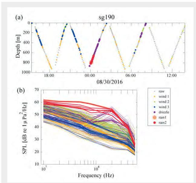
**Figure 7. a:** Seaglider (SG-190) profiles during a field experiment at 10°N, 125°W. **b:** Acoustic spectra of wind and rain were identified using rule-based algorithms. **Color dots in a** correspond to **color spectra in b** and indicate the detection of wind and rain according to various detection rules (wind 1-3, rain 1-2, and drizzle). SPL, sound pressure level; raw, no rain or wind.
