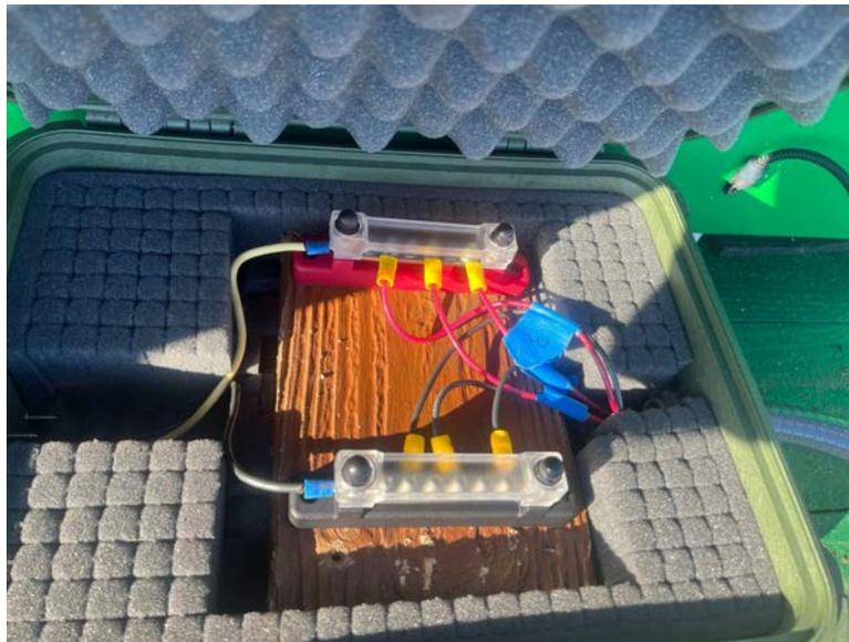
**Figure 25. Wiring for three bilge pumps.**
