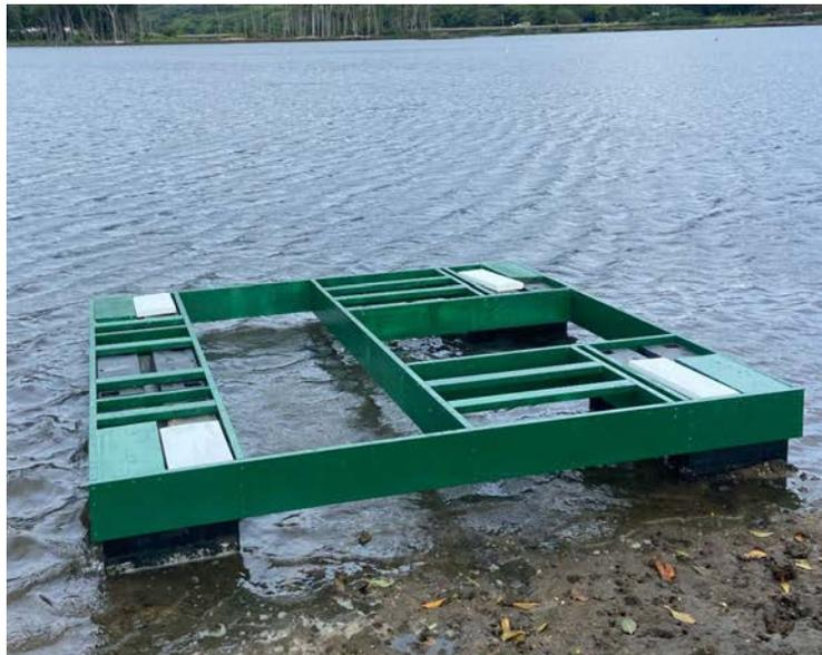
**Figure 20. Frame of the FLUPSY with dock floats.**
