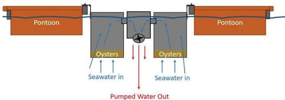
**Figure 4. Diagram illustrating a FLUPSY ( Pump Industry, 2023).**
