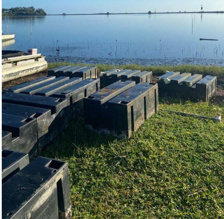
**Figure 19. Dock floats used in the construction of the FLUPSY.**
