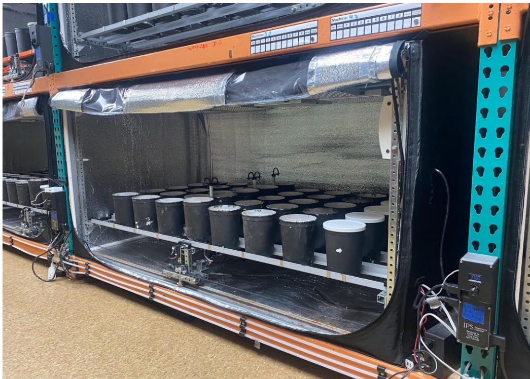
Figure 2: Picture of one of the Mora Lab Intelligent Plant Growing System (IPS) growth chambers with door open (Photo by author)
