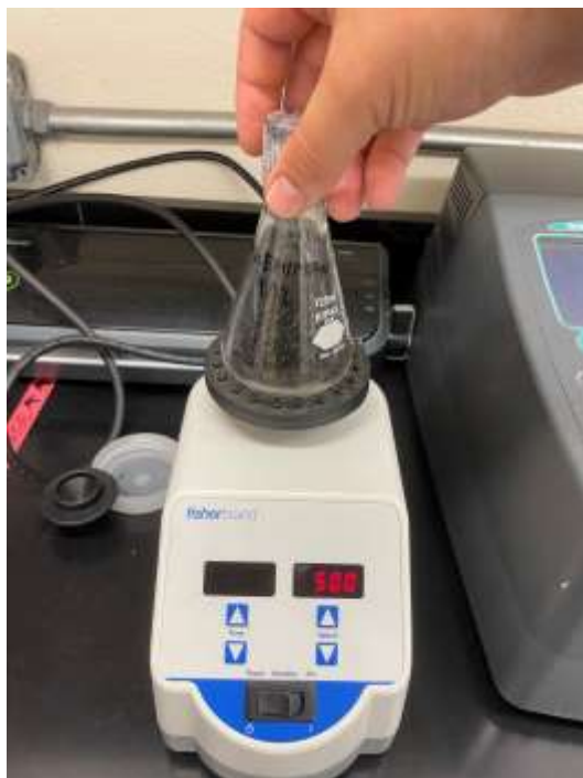
Figure 4: Vortex mixer aiding in agitation of sorbent onto activated carbon support. In the picture this particular impregnation was the Manganese [EMIM][OAc] sample.
