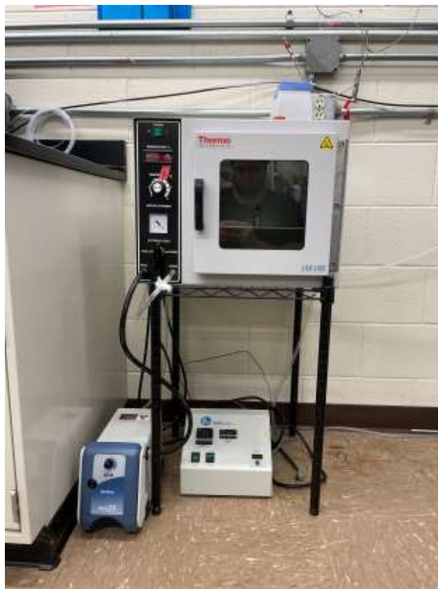
Figure 5: The vacuum oven is the equipment on the stand. The evacuation is operated through the pump located on bottom left (blue equipment).
