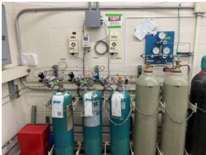
Figure 7: All gas cylinders used for this project from left to right: SO 2 concentration 188.7ppm, NO 2 concentration 200.7 ppm, H 2 S concentration 200 ppm, and the last two are the Ultra-Zero Clean Air.
