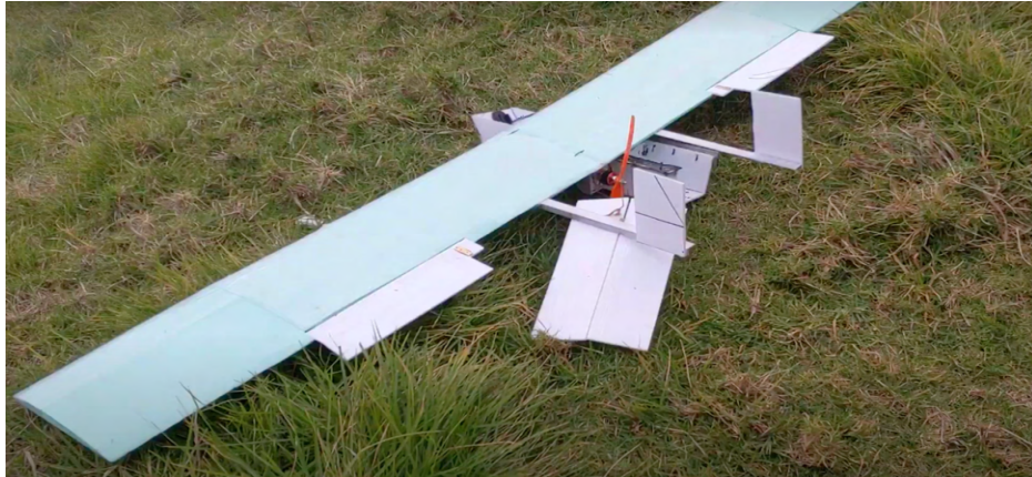
Figure 17: a) The Mk VI wing flexing to the point that the body detached from the wing mid-flight, b) Crash of Version 5 body on the Mark VI wing. Note the body is still fully intact, and only minor repairs were needed on the tail.
