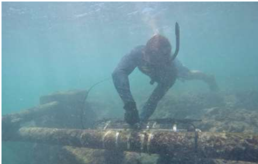
Photo courtesy of Shaun Wriston. Shaun servicing a Sea-Bird Electronics CTD sensor along O'ahu's south shore for the PacIOOS Nearshore Sensor Group. (Photo credit: Gordon Walker)
