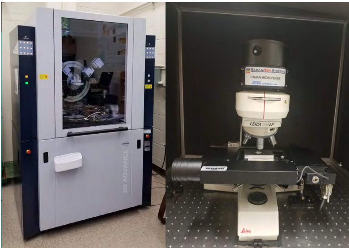
Fig. 4. Venture D8 XRD (Left) and Leica DMLP Raman (Right).
