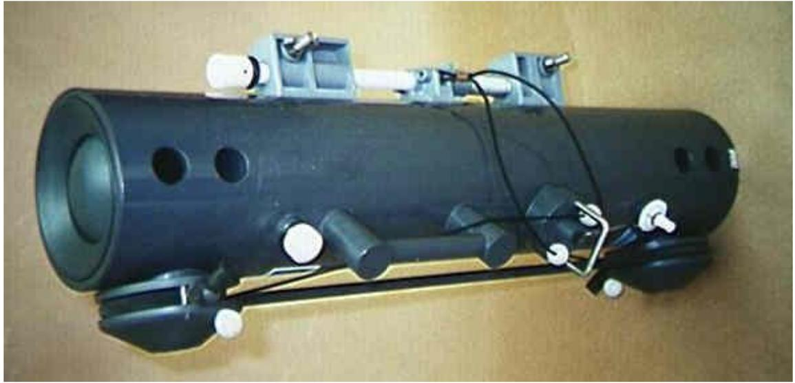
Figure 5: Picture of a Teflon-coated 30-l PVC ball-valve sampler courtesy of <http://www.act-us.info>.
