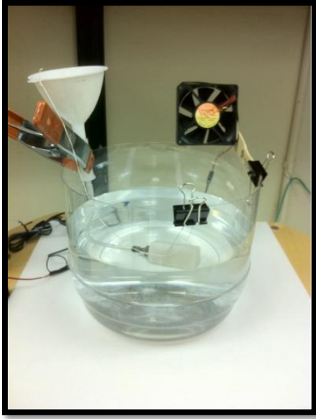
Figure 8: Pretzel Tank with Porous Rock on Water
