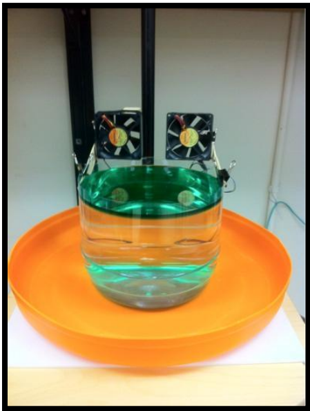
Figure 10: Pretzel Tank, Thin Stratified Layer, Two Fans Mounted Top View
