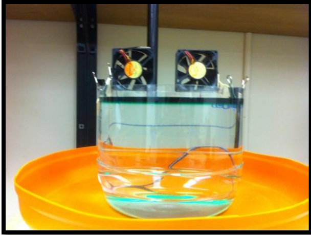
Figure 11: Pretzel Tank, Thin Stratified Layer, Two Fans Mounted Side View
