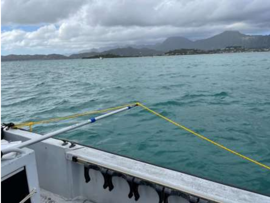
Figure 5: setup for plankton tow net. Rope was secured from cleat on bow to end of boathook to net 3-5m off of stern.
