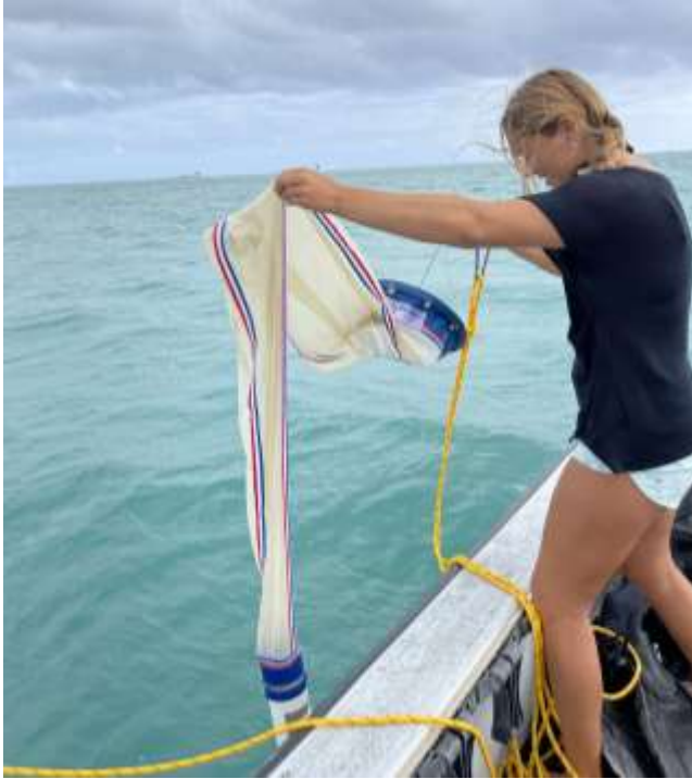
Figure 7: Retrieval and draining of the plankton net. Net was rinsed with seawater to ensure that all material collected was deposited into the collection cup, pictured at the base of the plankton net.
