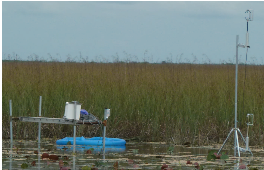
Figure 3.1: Platform, one limnocorral, and tripod with anemometers (85 cm and 3.0 m above water level) used in present experiment
