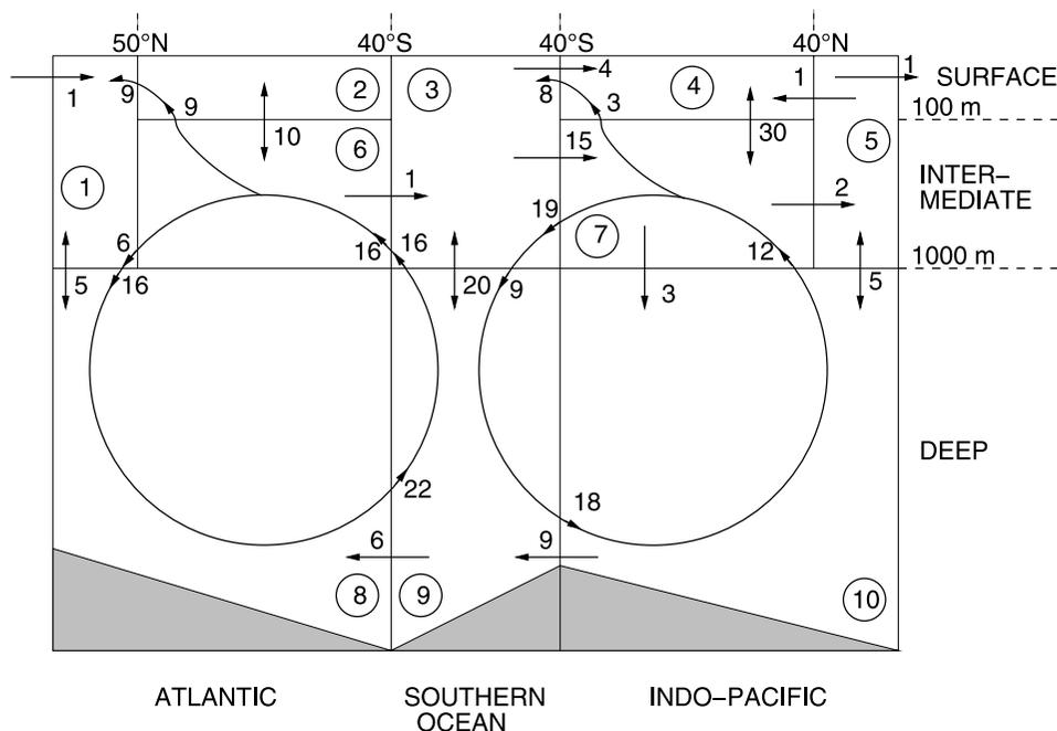
**Figure 2.** Geometry of the ocean box model and recent fluxes of ocean circulation (in  $\text{Sv} = 10^6 \text{ m}^3 \text{ s}^{-1}$ ). Box numbers are given in circles.
