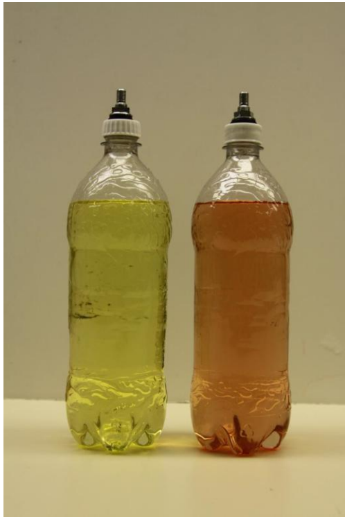
Figure 5.3: Demonstration of buffering using methyl red indicator dye. The bottle on the left contains saltwater and the one on the right contains freshwater.
