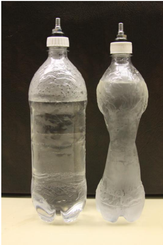
Figure 5.4: The bottle on the left contains warm water and the one on the right contains cold water. After removing all air from the headspace, the two bottles were filled with CO 2 and then shaken. Notice the difference in pressure between the two bottles.
