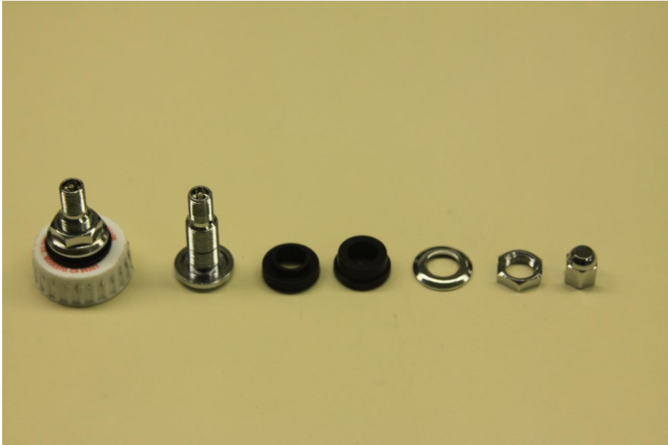
Figure 5.2: Pieces required for the bottle caps. The clamp-in tire valves can be purchased at an auto-parts store.
