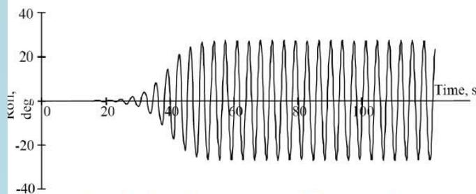
Figure 2.5: Example of parametric roll resonance [2]
