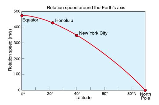
Fig. 2: The rotational speed of a point on the Earth's surface as it moves from the equator to the north pole.
