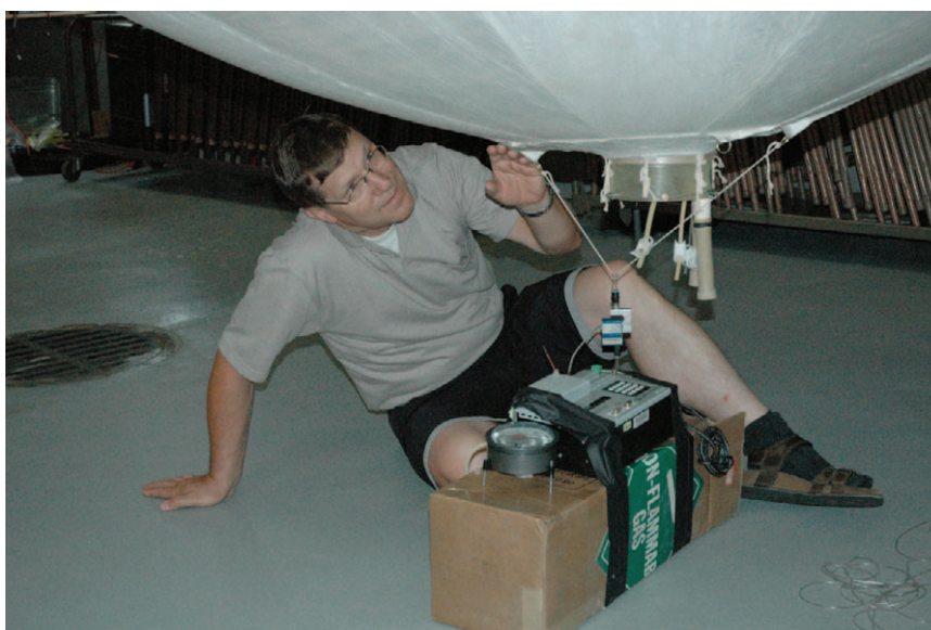
FIG. 9. NOAA's Randy Johnson, balloon engineer and designer, checks the superpressure of a smart balloon during ICARTT.
