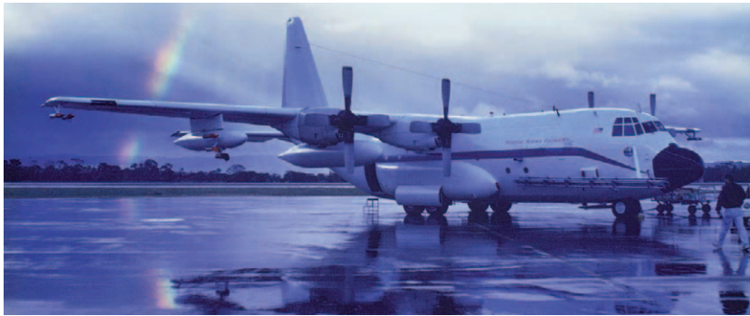
FIG. 5. The NCAR C-130 aircraft rests on the tarmac of the Hobart International Airport, in Tasmania, during ACE-I. When fully fueled, the NCAR C-130 can carry a payload of 13,000 lb, including instruments, scientists, and flight crew.
