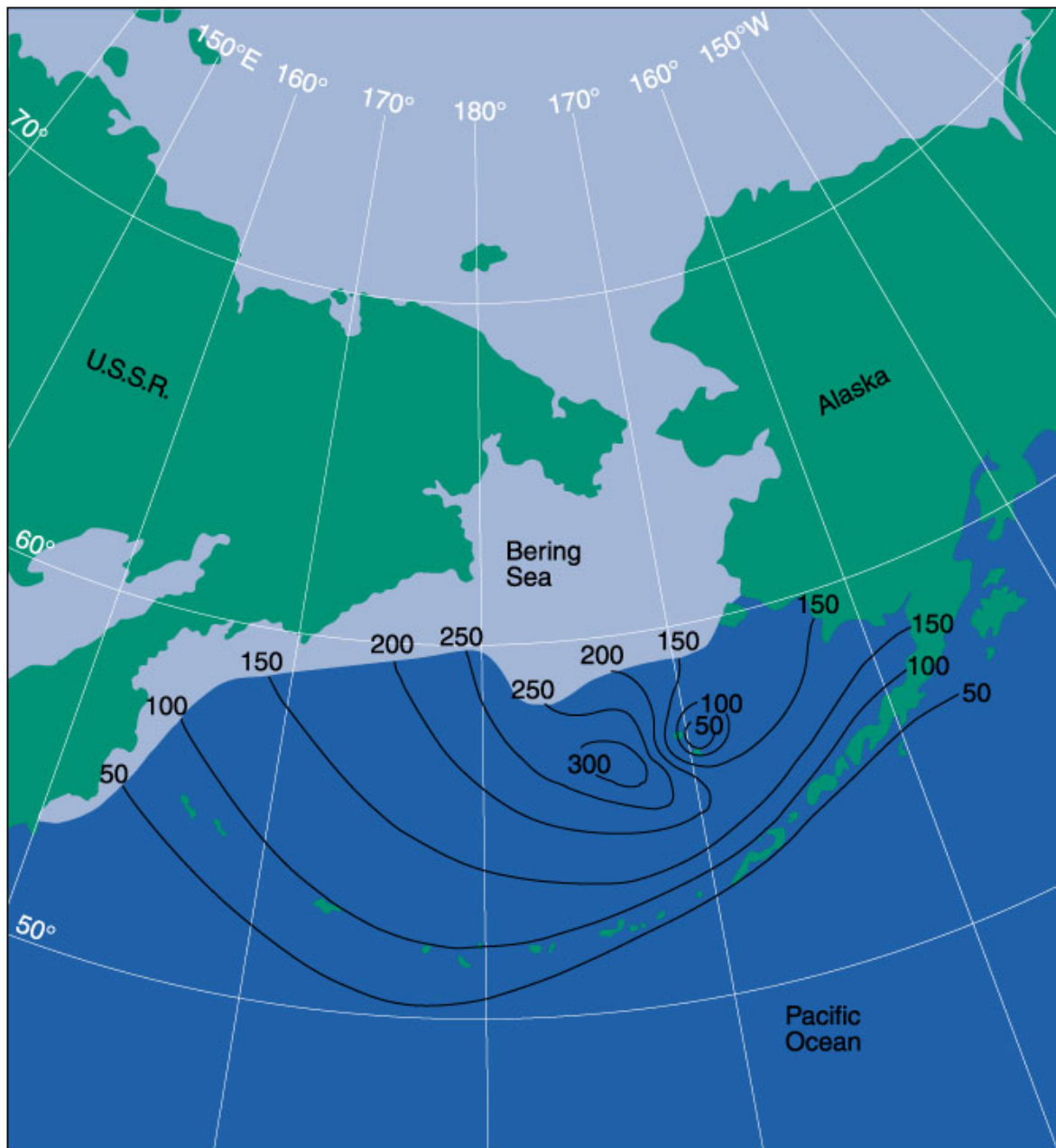
Figure 11. Sensible-heat fluxes—flows of heat from the ocean surface directly into the atmosphere—cause a perceptible warming at the core of an arctic hurricane. This warming, a result of the difference in temperature between air and sea, distinguishes these storms from both tropical hurricanes and midlatitude cyclones. As the mature arctic hurricane in the Bering Sea in 1977 passed over St. Paul Island (at 18:00 Greenwich Mean Time on March 8), these fluxes were greater than 300 watts per square meter in a tongue of arctic air just to the west of the surface low-pressure center. In the center itself, where the winds were light and the air had been warmed by previous surface heat transfer, the fluxes were small.
