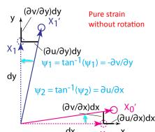
Shear strain > 0 if angle between +x and +y axes decreases
