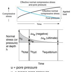
$u_e = \underline{\text{excess}}$  pore pressure
