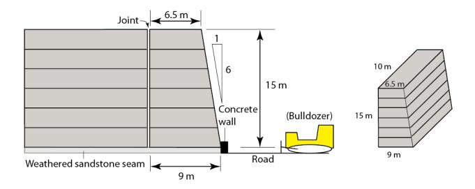
Case 2: Water rises to 10 m above the top of the weathered bed because the drainage in the concrete wall gets blocked.
