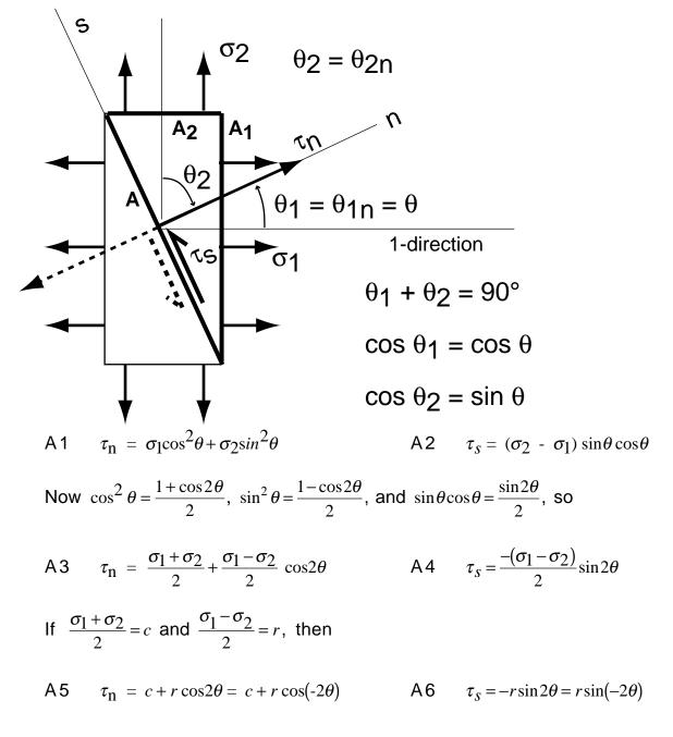
These are the equations of a Mohr circle for traction that relates the tractions on planes of different orientation at a point. Its center "c" is the mean normal stress (traction), and the absolute value of "r" is the magnitude of the maximum shear traction (the circle radius). The term  $\sigma_1$  is the most tensile stress.
