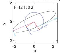
Vectors along axes of ellipse transform back to perpendicular vectors along axes of unit circle
