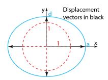
Position vectors that define a unit circle transform to position vectors that define an ellipse because [X'] = [F][X].
