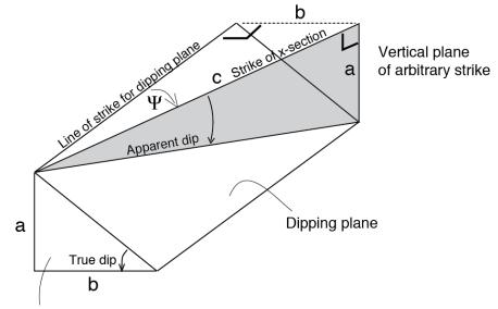
Vertical plane that is perpendicular to strike of dipping plane
