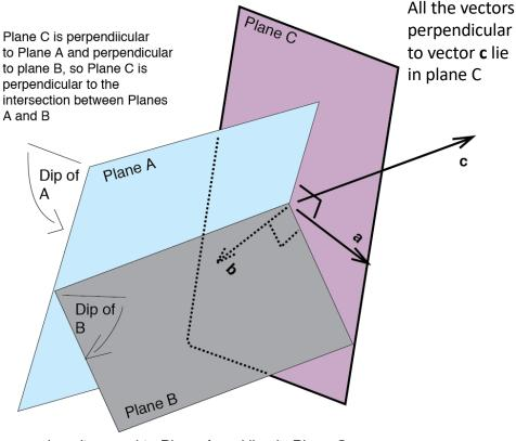
a is unit normal to Plane A and lies in Plane Cb is unit normal to Plane B and lies in Plane Cc is unit normal to Plane C
