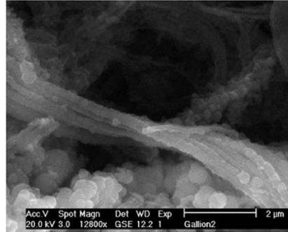
Figure 1: Hematite crystallites in and on stalks by Gallionella
