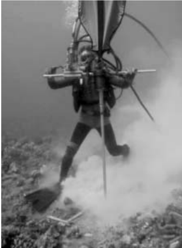
Research into the history of Hawaiian reef systems has been aided by development of our hydraulic rotary drill that can obtain 10-15 m cores. Former post-doctoral researcher John Rooney cores the fringing reef, south shore of Molokai.
