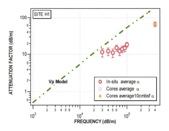
**Figure 8.6**Model simulations for site H1 intrinsic attenuation factor.
