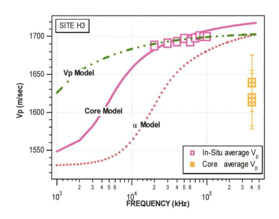
**Figure 8.3**Model simulations for site H3 compressional wave velocity.
