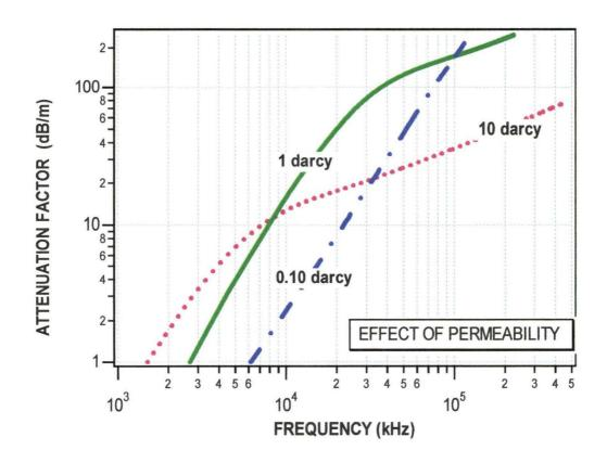
Figure 7.6  $\label{eq:Figure 7.6}$  Effect of dynamic permeability decreasing on intrinsic attenuation factor  $\alpha.$
