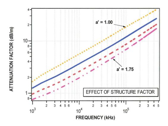
Figure 7.10  $\label{eq:figure 7.10}$  Effect of structure factor increasing on intrinsic attenuation factor  $\alpha.$
