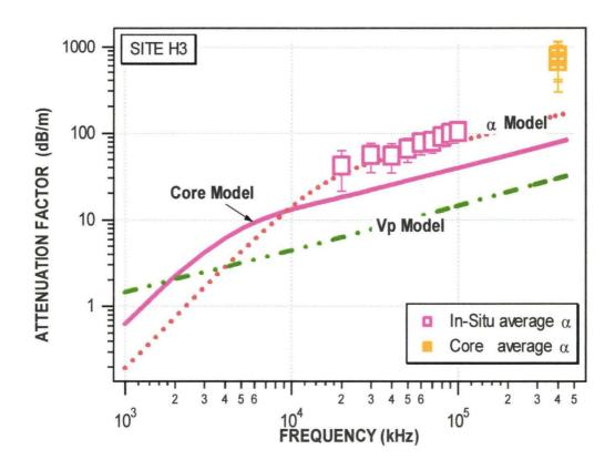
**Figure 8.4**Model simulations for site H3 intrinsic attenuation factor.
