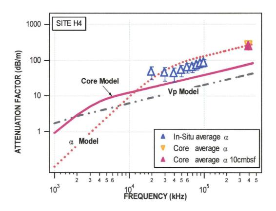
**Figure 8.2**Model simulations for site H4 effective attenuation factor.
