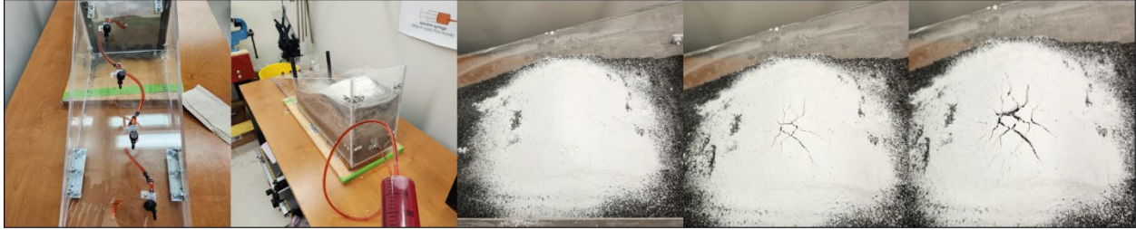
Fig. 25. Sequence of photos show (from left to right) the faucets of the system closed, while red water is being injected creating radial cracks at the summit of the modeled volcano.
