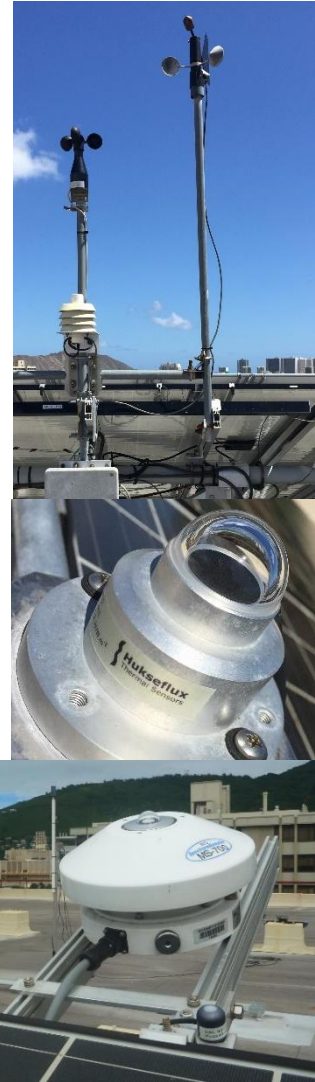
Figure 2 – Parts of the weather station (top), thermopile pyranometer (middle), masked pyranometer (bottom left), and spectroradiometer (bottom right).
