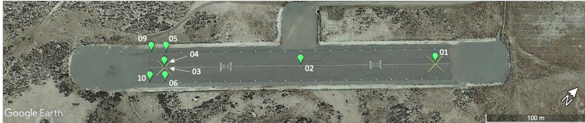
Figure 1. Smartphone layout for UAV test flights. Smartphone positions are indicated with green placemarks and numbers correspond to the station ID of each smartphone.
