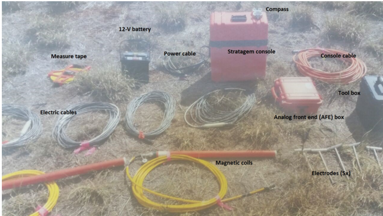
Figure 5: AMT equipment used for measurements.
