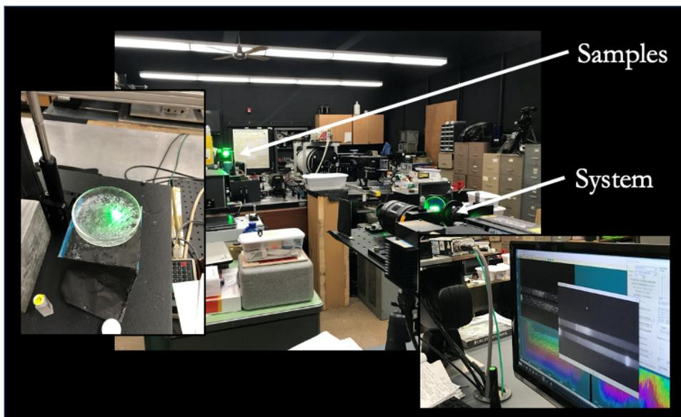
**Figure 3.3:** A compilation of images showing the experimental setup. On the left is a zoomed in image of a sample being measured. On the right is an example of the ICCD image output when measuring a target.
