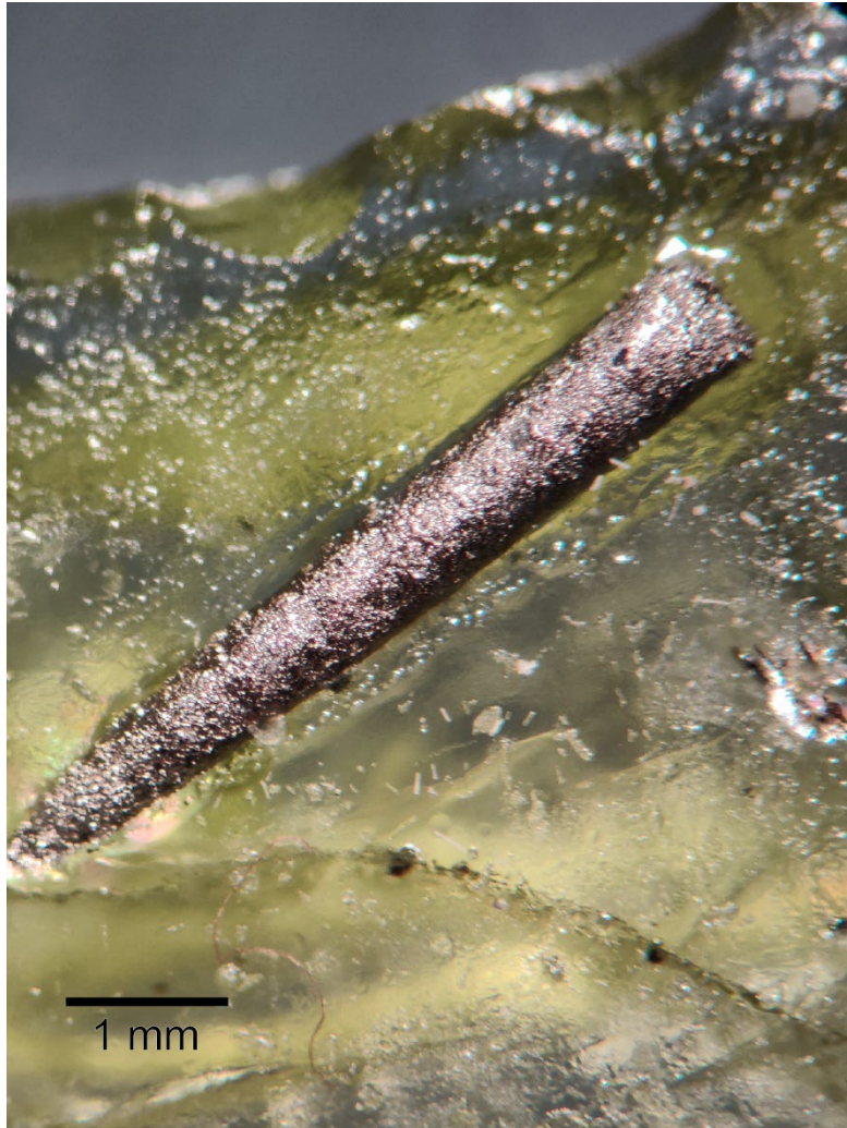
Figure B-3: Initially pure Pt wire after 10 days on SCO at 1400 °C. The wire has bore ~25 microns into the olivine here, and has become 11.5 wt% Fe.
