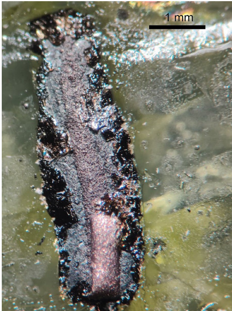
Figure B-2: Pt wire with 59.8 wt% Fe after 10 days on SCO at 1400 °C. Notice a substantial amount of oxides have grown around the wire.
