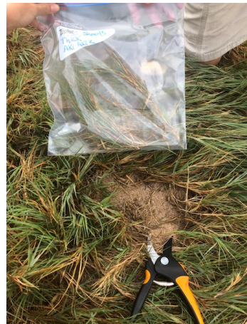
Figure 18. Cutting 'Aki'aki shoots before using the hand auger to core into the ground.
