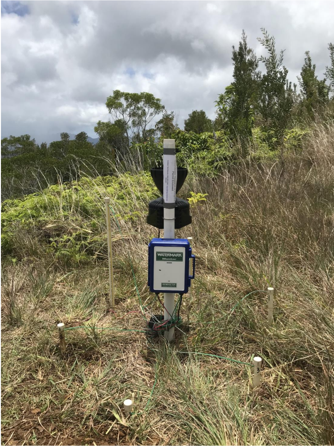
Figure 4. Upper Manana study with five soil tension probes, a tipping bucket style rain gauge, a soil temperature probe, a cumulative bulk precipitation collector (not shown), an Irrometer 900M data logger, and an OnSet Computer Corporation HOBO U14-001 Temp/RH Data Logger.
