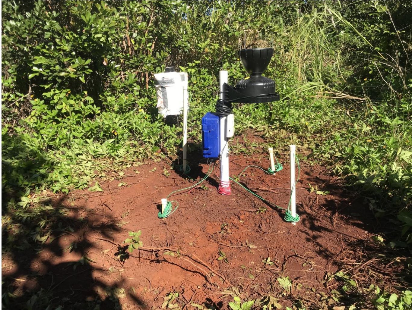
Figure 3. Lower Manana study site with four soil tension probes, a tipping bucket style rain gauge, a soil temperature probe, a cumulative bulk precipitation collector, an Irrrometer 900M data logger, and an OnSet Computer Corporation HOBO U14-001 Temp/RH Data Logger.
