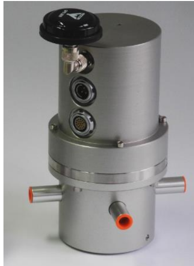
Figure 1.3. MB3 digital microbarometer (MB3d); a digital infrasound sensor designed to meet IMS specifications. The sensor consists of a transducer block (bottom) with an aneroid capsule coupled with a magnet-and-coil transducer. A secondary coil wrapped around the main one ensures remote calibration capability. The second block of the sensor is the digitizing block (top), which samples the analog output of
