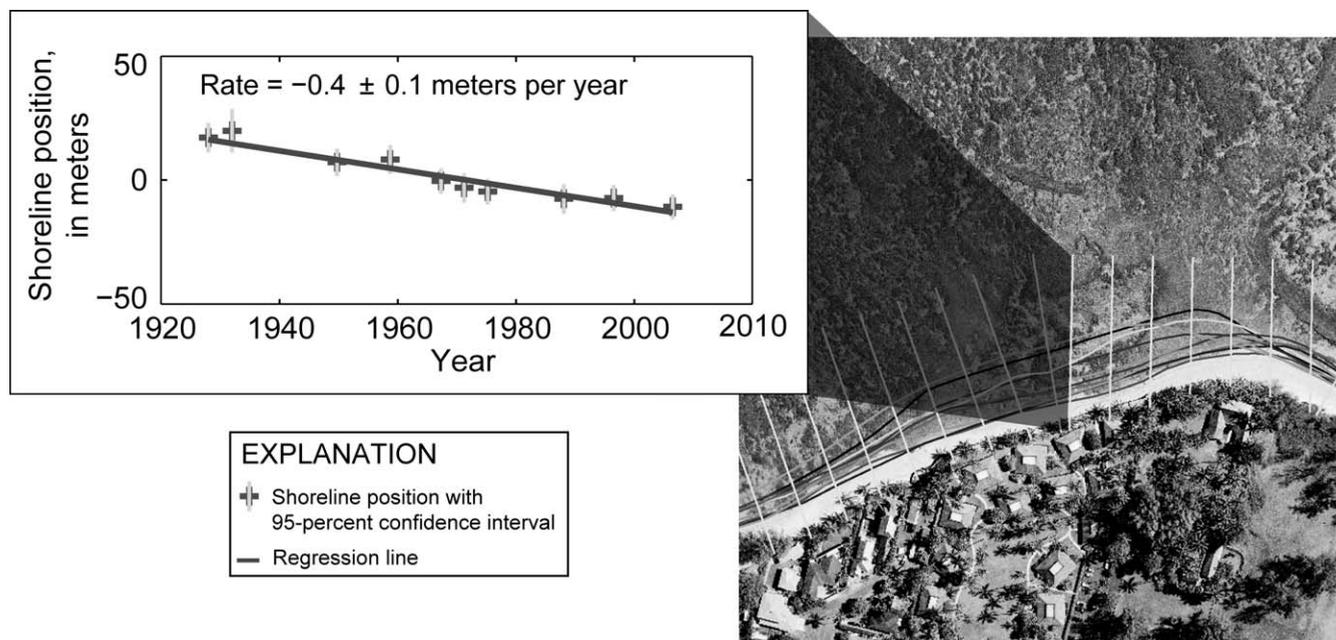
Figure 3. Historical shorelines (shore-parallel lines) are measured at regularly spaced transects (shore-perpendicular lines, ~20 m spacing). Shoreline change rates are calculated using weighted least squares (WLS) linear regression (Fletcher *et al.*, 2012).
