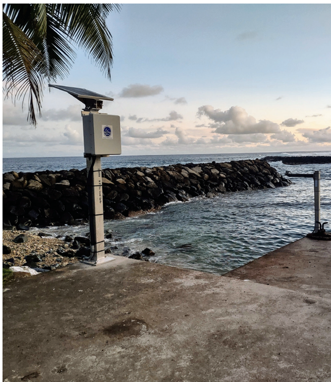
(above) New UHSLC tide gauge in the village of 'Au'asi on Tutuila Island, American Samoa. Photo Credit: Jason Klem.
