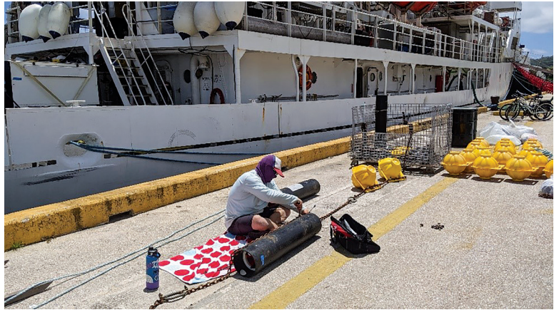
(above) Erik Norris assembles a HARP for deployment off Saipan. Photo credit: Yvonne Barkley.
