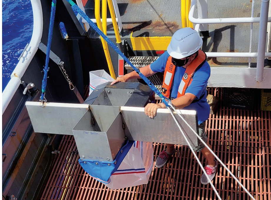
Testing of a high-speed mini surface trawl designed and fabricated by the Marine and Applied Knowledge for Ecosystem Research Laboratory (MAKER Lab) on the Big Eye Tuna Research Mission aboard the NOAA R/V Oscar Elton Sette. Photo Credit: Johanna Wren.
