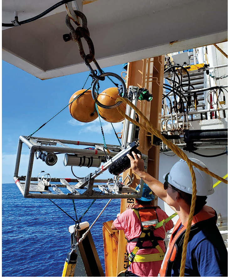
Recovery of the MOUSS camera system with green led lights on R/V Oscar Elton Sette during the SE-22-07 Bottomfish cruise. Photo Credit: Christopher Demarke.
