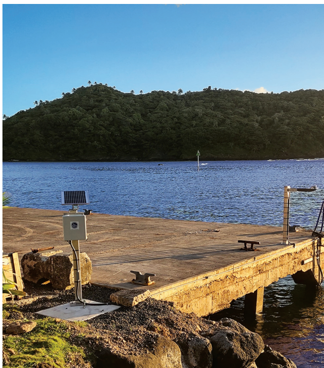
(below) New UHSLC tide gauge on Ofu, part of the remote Manu'a Islands of American Samoa. Photo Credit: Jason Klem.
