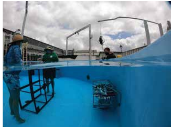
Figure 4. Calibrating Modular Optical Underwater Survey System (MOUSS) prior to 2021 Bottomfish Fishery-Independent Survey in Hawai'i (BFISH) operations. Photo Credit: Kyle Koyanagi.
