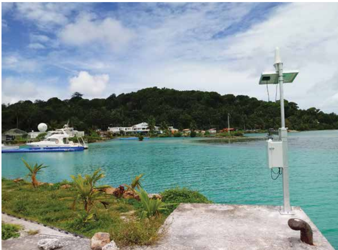
Figure 1. Photo of the new UHSLC tide gauge installed on Chuuk, Federated States of Micronesia. This gauge was installed via remote collaboration during the COVID-19 pandemic with colleagues at the Korea-South Pacific Ocean Research Center on Chuuk. Photo Credit: Korea-South Pacific Ocean Research Center (KSORC).
