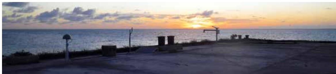
Figure 1. Sunset view of the new Global Navigation Satellite System (GNSS) site “JSTN” installed on Johnston Atoll on May 24th 2021 as part of the effort to install GNSS sites at all tide-gauge stations within the Global Sea-level Observing System Core Network. The photo shows the GNSS antenna at the bottom left. To the right of it are the instrument box, the Iridium satellite communications antenna, the solar panel (next to two unused bollards), and the tide gauge. The GNSS provides high-accuracy vertical positions and velocities in the global reference frame. The GNSS antenna is surveyed as part of the tide gauge leveling network, and the vertical offset between it and the tide gauge reference level is precisely measured. Photo credit: Jason Klem.
