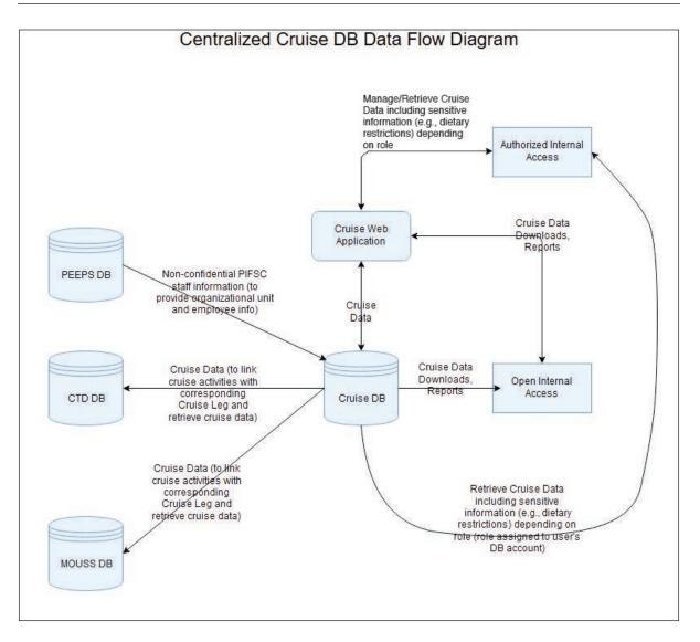
Figure 2. Formal data flow diagram for the current version of the CCD showing how it relates to other enterprise database schemas.
