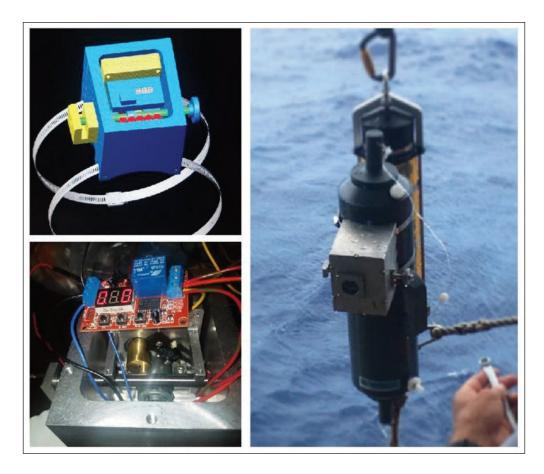
Figure 3. A custom designed and fabricated eDNA Niskin bottle release for collecting water samples at a depth of ~250 msw in association with DropCam Instrument Package rigging (DCIP). Top left: release design concept. Bottom left: electronics fabrication. Right: shown attached to the acoustic release of the DCIP after successful implementation in the field.
