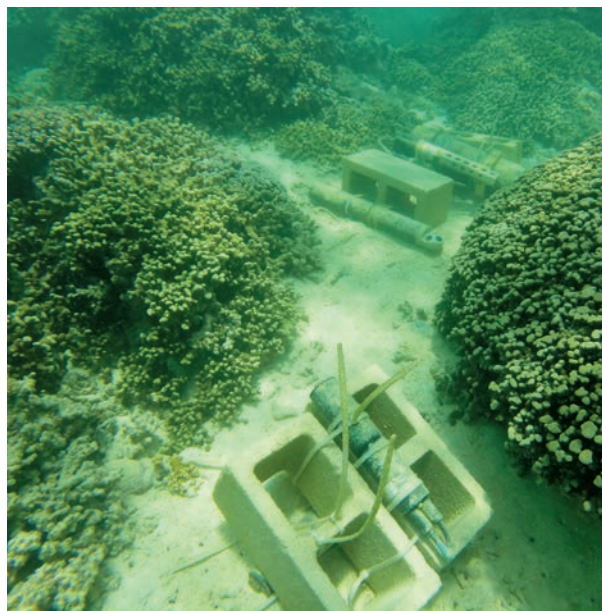
Figure 1. Instruments deployed on the seafloor in Kaneohe Bay, Oahu, Hawaii, between coral heads as part of an evaluation of capabilities for high endurance automated measurements of inorganic carbon system parameters.
