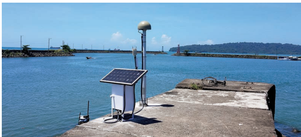
Figure 1. The newly installed continuous GNSS site "CILI" at Cilacap, Indonesia. The previous tide-gauge and GNSS site had to be moved due to demolition and construction at the old location. The tide gauge is about 200 m to the left.
