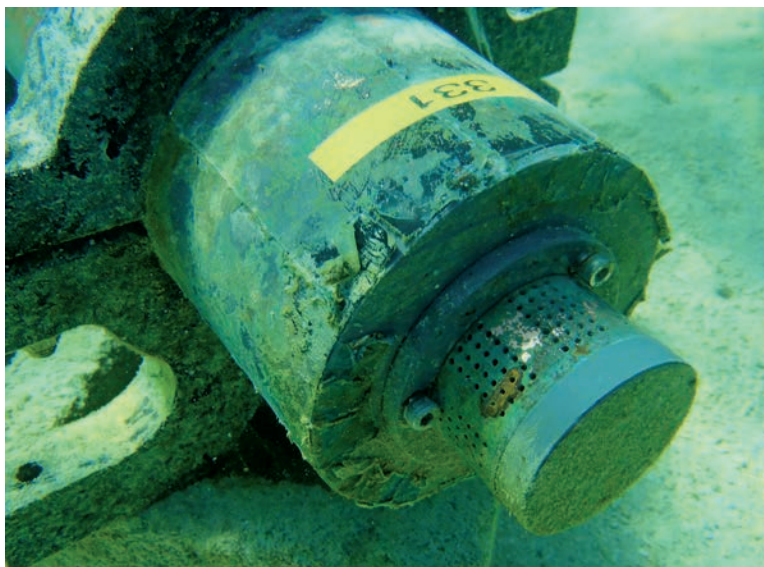
Figure 2. Close up of a SeaFET pH sensor showing evidence of biofouling.
