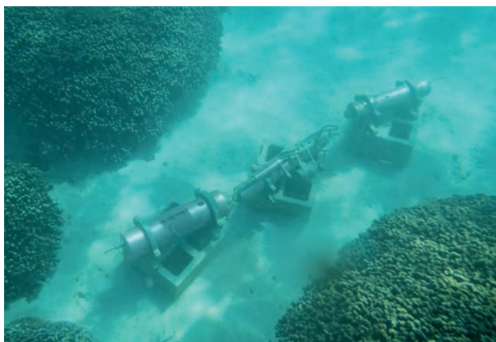
Figure 1. Set of three different sensors deployed on a sandy patch between coral heads adjacent to the CRIMP-2 buoy on the barrier reef of Kaneohe Bay, Oahu, Hawaii
