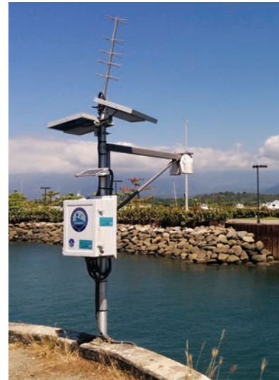
Figure 1. UHSLC tsunami water level station at Quepos, Costa Rica.
