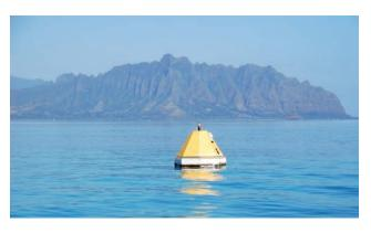
Figure 1. The CRIMP-2 MAPCO<sub>2</sub> buoy has been making automated measurements of inorganic carbon system parameters on the barrier reef of Kaneohe Bay, Oahu, Hawaii since June 2008. Kualoa Point, a spur of the Koolau Range can be seen in the background.
