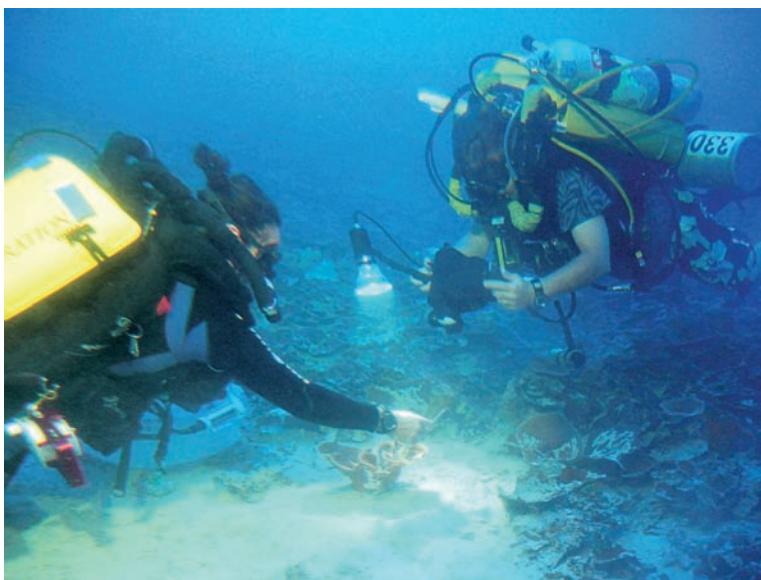
Figure 1. Scientists using closed circuit rebreathers and mixed gas measure work in combination with the Hawaii Undersea Research Laboratory's Pisces V submersible to photograph, measure, and stain a coral colony for growth rate studies. The use of combined technical scuba and research submersible dives was pioneered during cruise KOK11-02. (Photo: John Rooney)
