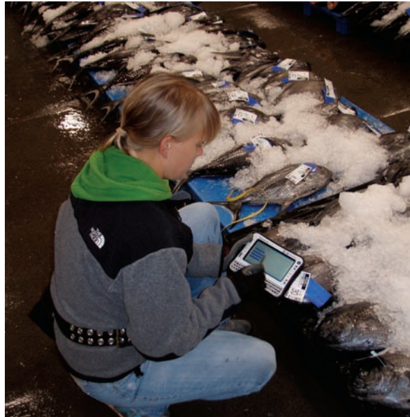
Figure 1. Fisheries associate sampling pelagic fish species at the UFA fish auction using the toughbook barcoding system designed specifically for the Life History program.
