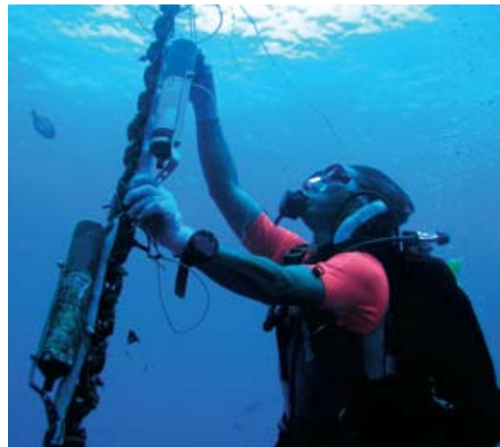
Retrieving an acoustic data logger from a FAD
