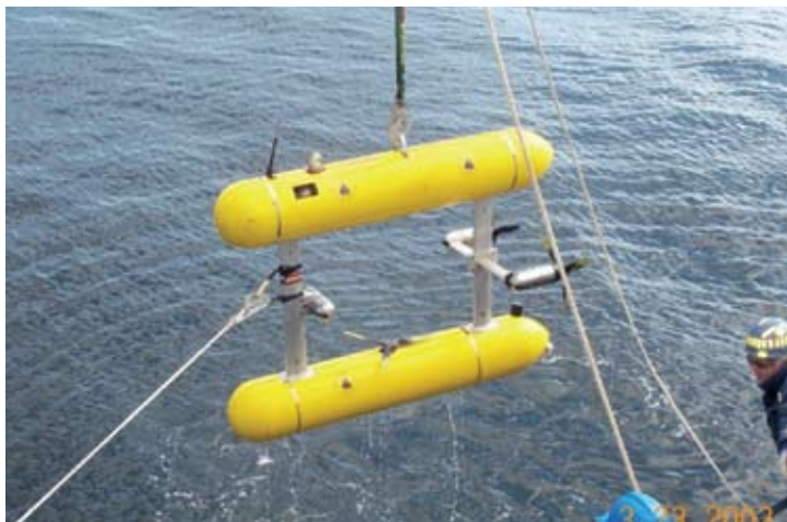
In partnership with the Northwest Fisheries Science Center and Woods Hole Oceanographic Institution (WHOI), CRED participated in three training and field operations using a newly acquired SeaBED AUV. This vehicle enhances the photographic and video mapping of coral-rich environments, providing data in a greater range of depths and more effectively than do towed vehicles attached to a surface vessel. Courtesy: WHOI Deep Submergence Laboratory
