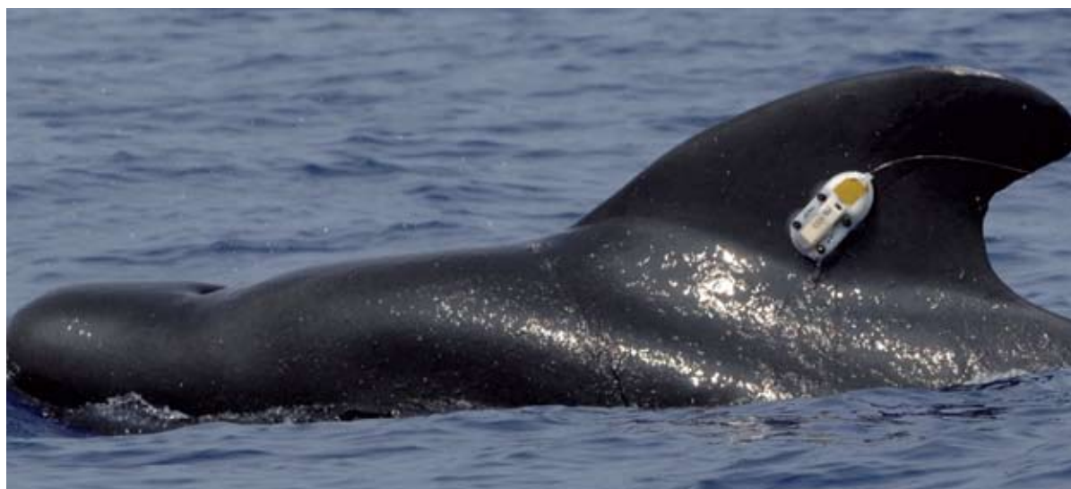
Pilot whale carrying a Digital acoustic recording tag (DTAG) during the RIMPAC08 collaborative survey off the Kona coast of Hawai'i.
