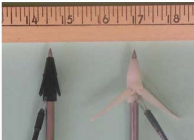
Figure 1. Picture of the two dart types; the black umbrella dart and the large white dart. The white dart appeared to increase the duration of tag deployments.
