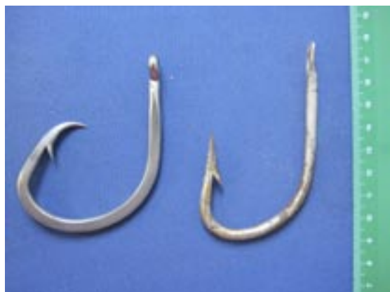
(top) Hooks used in experiment. Left—18/0, 10° offset circle (“C”) hooks; Right—Portuguese style 9/0 stainless steel (“J”) hooks. (Photo A. Domingos). (bottom) Loggerhead sea turtle caught in longline fishing gear in Uruguay. (Photo C. Barcelo).
