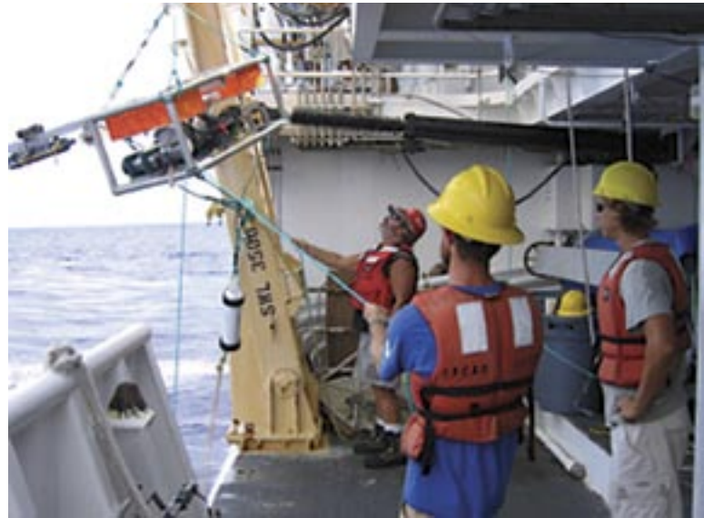
JIMAR researchers prepare to deploy the Bottom fish camera (BotCam) station in waters off the Commonwealth of the Northern Marianas Islands. The BotCam is a non-extractive method to collect information about bottom fish species in depths up to 350 meters.
