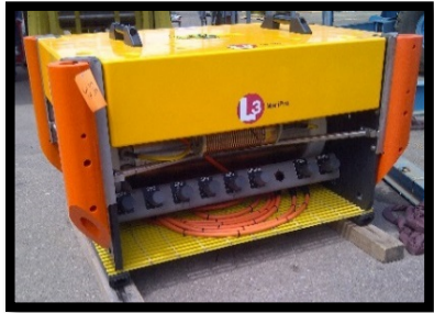
Cabled Array ROV Serviceable Node
