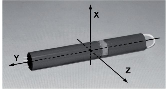
**Fig. 1.** Diagram of the XYZ acceleration logger showing the orientation of all three acceleration sensors (X, Y, and Z respectively). Courtesy of VEMCO (Nova Scotia, Canada).
